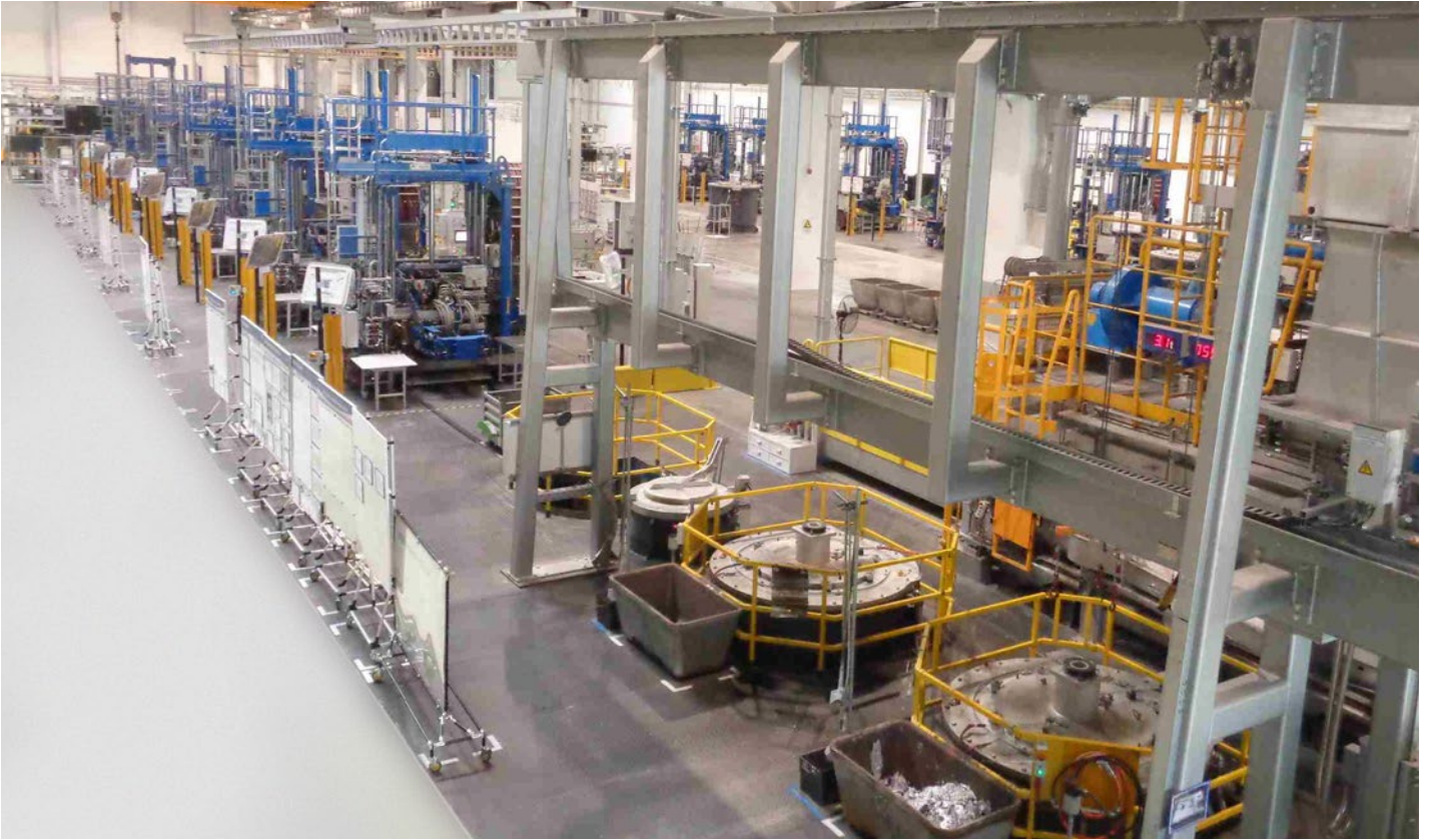
Turnkey foundry for the production of engine blocks at BMW Brilliance Automotive in China
