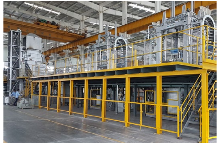
Casting line with platform, holding and degassing station for the production of structural parts
