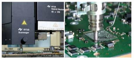
Left: Auto Scavenger module of the HR 600 XL for non-conact residual solder extraction. Right: After the component has been automatically lifted off the PCB, remaining solder is removed completely.
