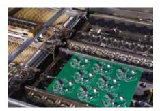
The vacuum module's roller conveyor is free of lubricants.
