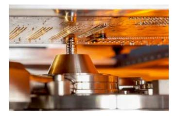
The innovative "Peel-Off" function of the Ersa mini wave soldering modules in single solder pots enables to optimally form solder joints when soldering on a horizontal level, and the formation of solder shorts (bridging) can be almost eliminated. Since there is no preferred direction in the run-off of the solder from the nozzle, the solder wave can be moved in any direction.
