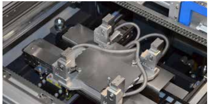
Fluxer unit with 4 spray heads
