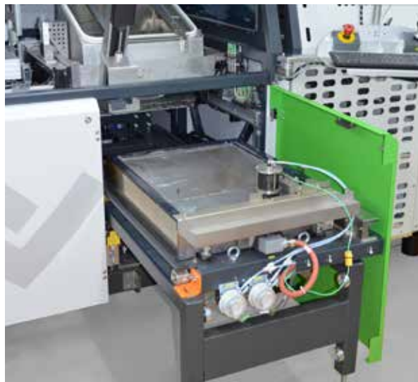
Solder bath in maintenance/set-up position
