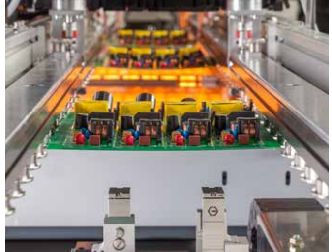
Multidrop precision fluxer: Highest process safety through flux volume measurement and control
