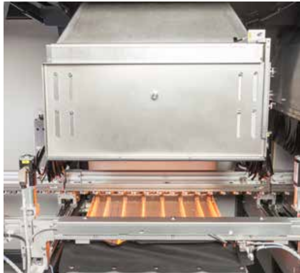
Power convection for a homogeneous through warming of the PCB – even for the most complex boards
