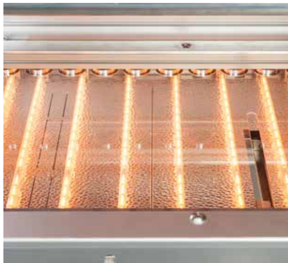
Bottom-side preheater cassette – IR emitters can be switched in groups
