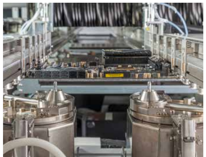
Dual pot system, Y axis variable, Z axis fixed
