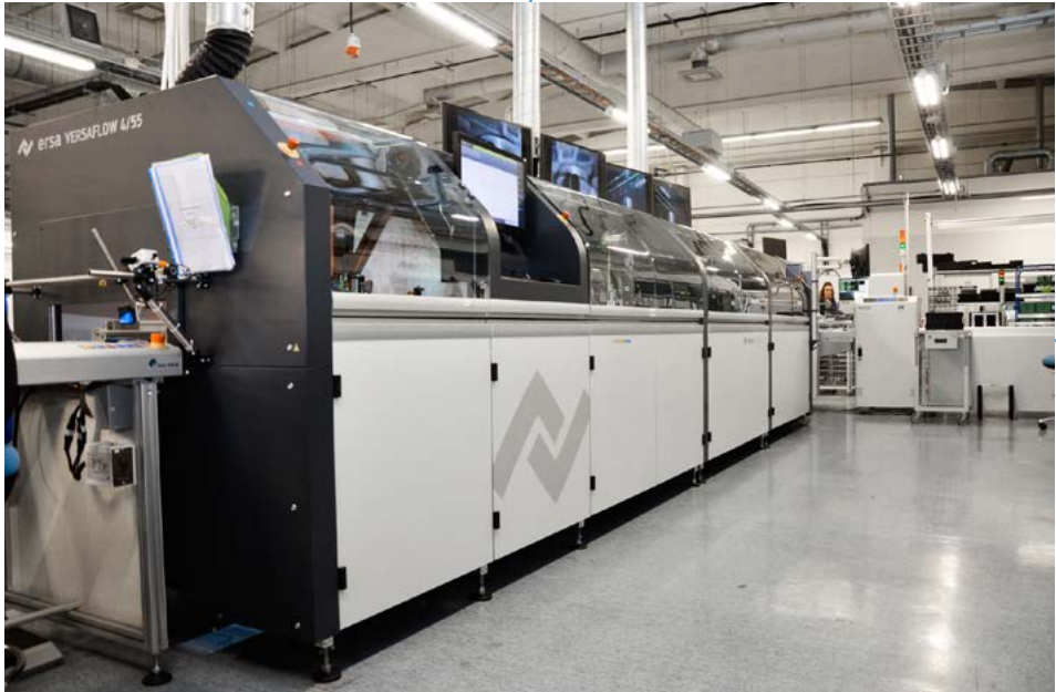
Ersa selective soldering system VERSAFLOW 4/55 with VERSAFLEX in the Kitron production in Kaunas.
