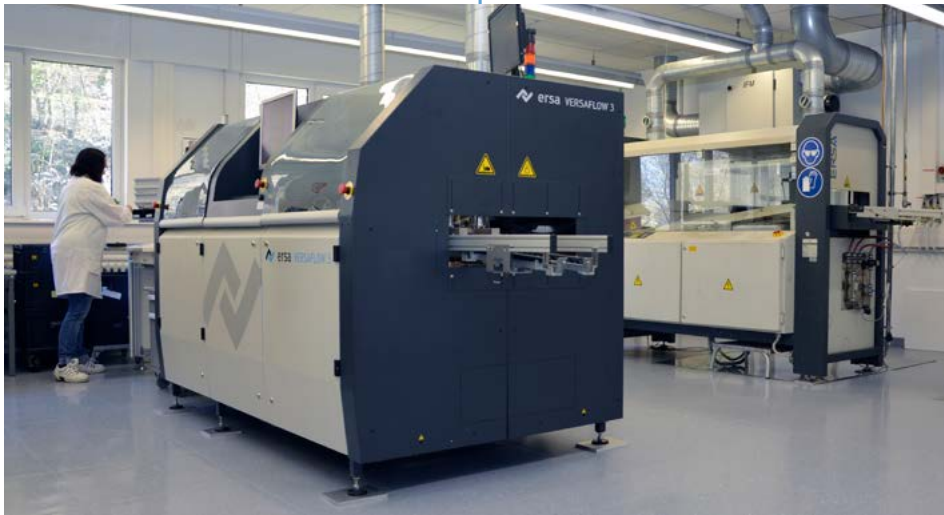
With two pots, ideally equipped for the highest-possible throughput: ErsafLOW 3/45 in the HUND manufacturing process.
