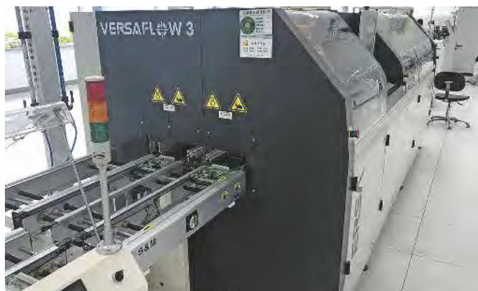
The Versaflow 3/45 selective soldering system with dual track.
