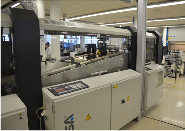
Existing wave soldering line ERSA N-WAVE 330 at the Variosystems Steinach site near Lake Constance.
