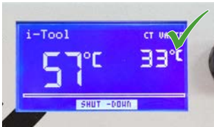
Use soldering station shutdown
