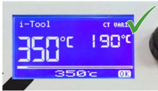
340 – 360 °C for lead-free solder (644 – 680 °F)
