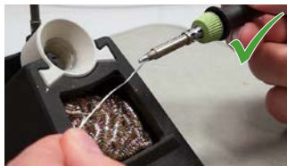
Add new solder after cleaning
