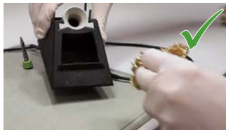
Remove dirty metal wool and empty the solder collecting box
