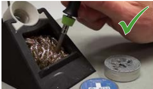
Clean from tip reactivator residues
