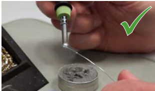
Add new solder after cleaning
