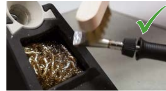
Alternative method: Clean by brass brush (3ZT00051)
