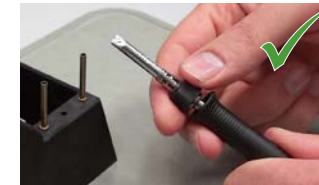
Switch off station, unscrew tip
