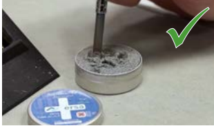
Stick wettable area of the tip into the reactivator paste (OTR02/SB) and move slightly
