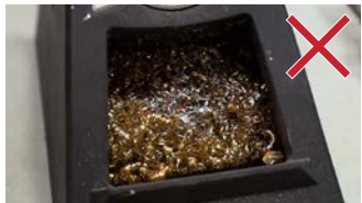
Dirty dry cleaner (flux and oxides)
