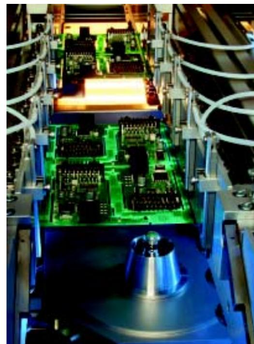
at completely eliminating the need for any form of dedicated, expensive tooling. The bottom-viewing camera allows us to verify machine setup in rapid fashion. Speed is, of course, a vital element where high-mix contract manufacturers are concerned.
