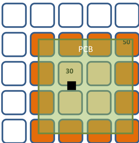
Figure 2.1 5 x 5 bottom heater matrix
