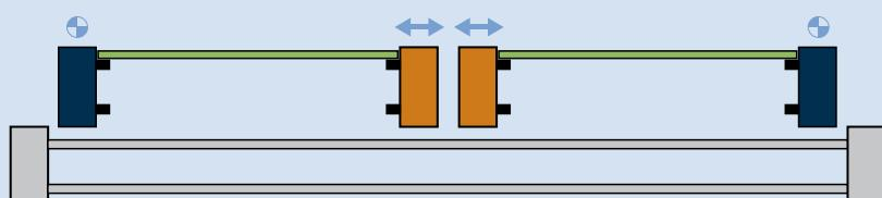
*As an alternative to the center supports, the conveyors could also be equipped with a low mass tubular support safety conveyor running below the conveyor rails (example shows safety conveyor below dual track conveyor).*
