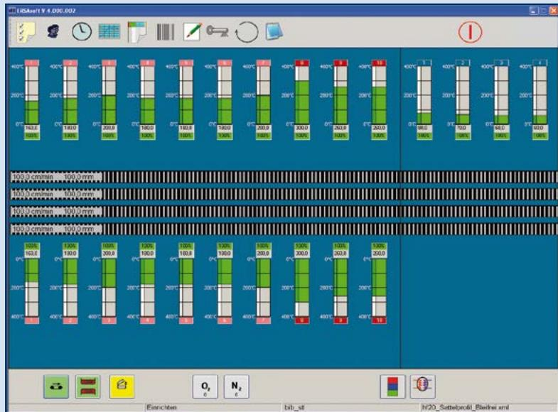
All Ersa reflow systems are operated under PC control with ERSASOFT. This machine visualization software offers numerous functions which assist the system user to operate the system error free.
